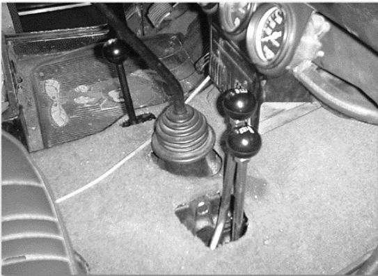
Twin sticks through modified hole in floor.
