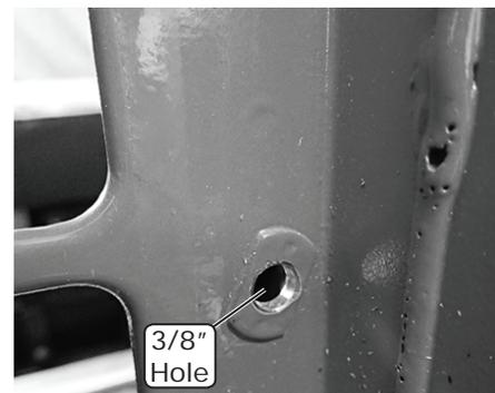
**NOTE: The weld nut will be removed while enlarging the hole.**
