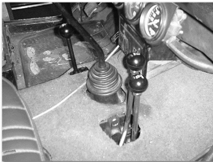
Twin sticks through modified hole in floor.
